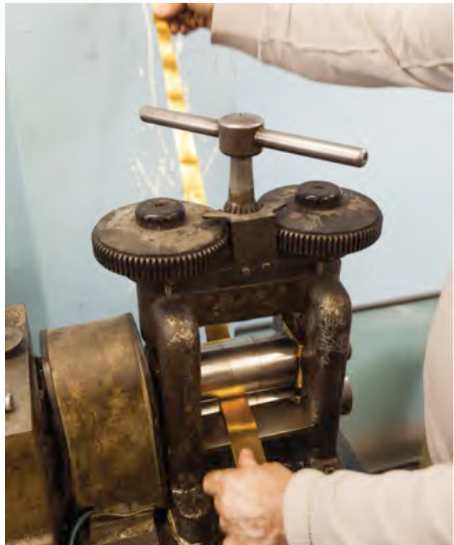
24ct gold is flattened into sheets in jewellery production.
